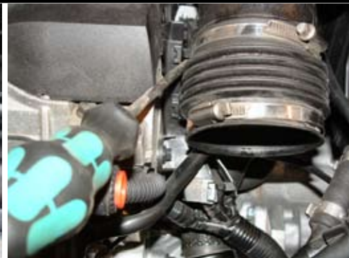
9. Cars with automatic gear box: Open the electrical harness cover.
