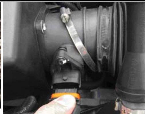
3. Disconnect the battery. Release the connector from the air mass meter and remove the inlet hose.
