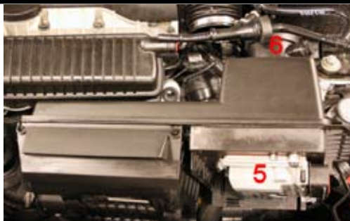
5. Pull the airfilter box rakt upwards until it releases from the rubber holdings, pull the box to the right and at the same time turn it to release the box. Remove the ECU (5) an the air mass meter(6) from the air filter box. (The rubber seal should not be used again.)
