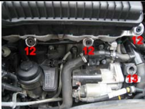
8. Assemble the plastic "washer" to the rubber bushings (12).
