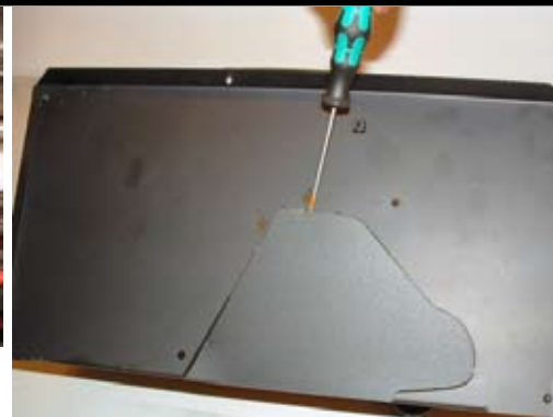
6. Remove the pre cut plate from the OptiFlow heat shield. Start with breaking the upper attach point, then wiggle the plate back and forward until it has come loose.
