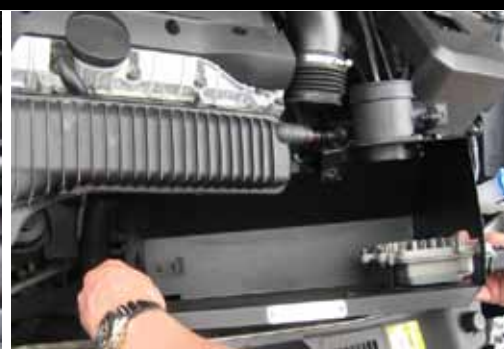
12. Assemble the OptiFlow heat shield to the car, slide it down from right to left. Fit the steering pin under the OptiFlow heat shield to the rubber bushing (See picture 11, point 13).
