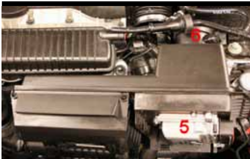
7. Pull the airfilter box rakt upwards until it releases from the rubber holdings, pull the box to the right and at the same time turn it to release the box. Remove the ECU (5) an the air mass meter(6) from the air filter box. (The rubber seal should not be used again.)
