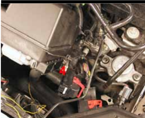
4. Remove the connectors (4) from the ECU. Loosen both of the red clips and pull the connectors.
