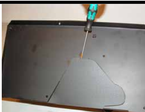
8. Remove the pre cut plate from the OptiFlow heat shield. Start with breaking the upper attach point, then wiggle the plate back and forward until it has come loose.
