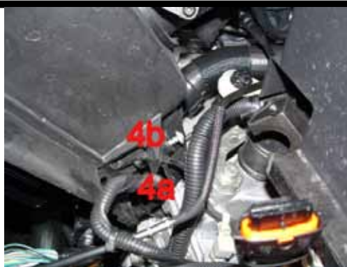
5. Remove the cable harness from the air filter box. Cut of the tie wrap (4a) holding the harness. Remove screw (4b).
