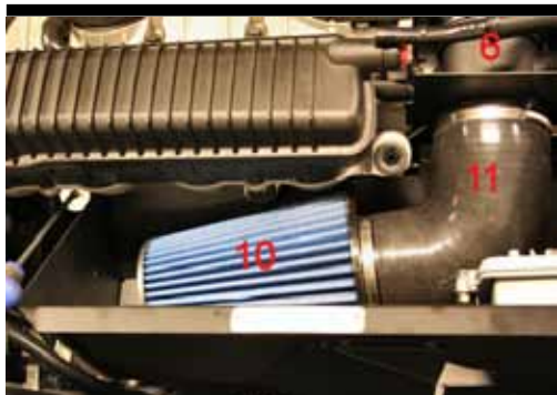
13. Do not tighten the screws to the heatshield yet. Assemble the air mass meter (6) BSR performance air filter (10) BSR intake hose (11). Now tighten the heat shield, start with the two attach points to the left, leave the third for later.
