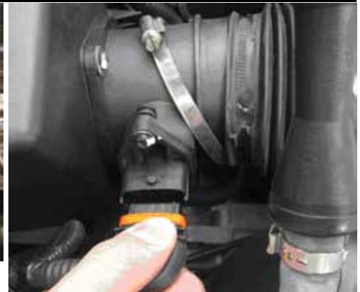
3. Disconnect the battery. Release the connector from the air mass meter and remove the inlet hose.
