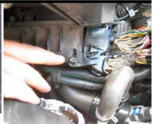
6. Remove the cable harness from the air filter box.
