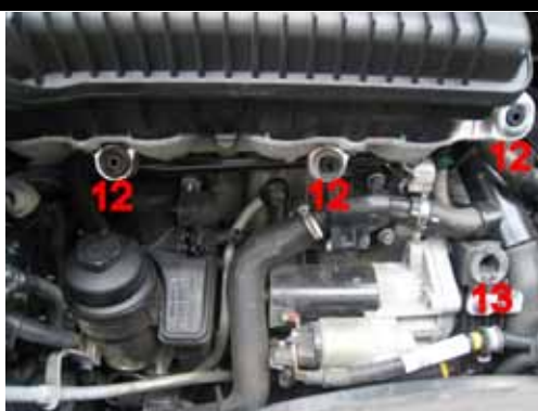
11. Assemble the plastic "washer" to the rubber-bushings (12).
